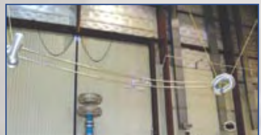
Electrical Corona Testing of VORTX Damper
